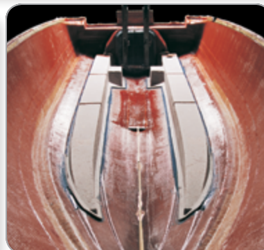
Bonded Fiberglass Stringers
