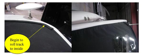
12. Butt an 81" piece of track to continue to the bottom of the arch.
