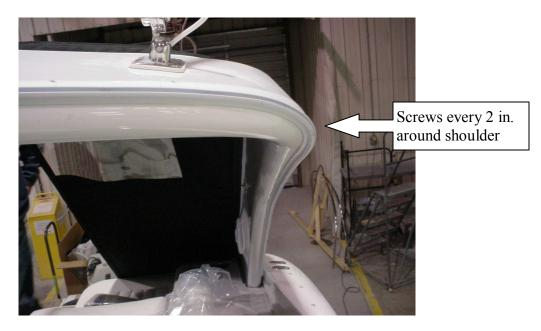
9. Use a 35" piece of track to continue the installation to bottom of the exposed arch.
