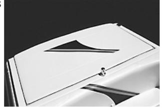
The storage of the boats' battery is located under the rear hatch. If the battery becomes discharged you will need to attach jumper cables to the battery post terminals located on the port side of the rear passenger seat to restart. You cannot open access hatch if battery is dead unless power is supplied to the battery.
