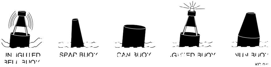
Figure 1-7. Buoy Shapes
