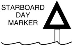
Day markers are colored and numbered the same as buoys. RED, triangular day markers with even numbers mark the starboard side of the channel. GREEN, square day markers with odd numbers mark the port side of the channel.
