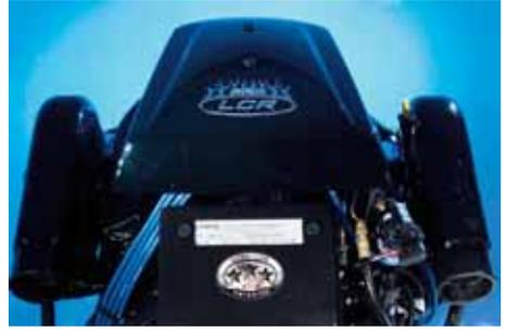
Figure 4-5. 5.7L LCR Engine
