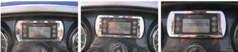
3. Make sure the Wedge is all the way down before you proceed. Make sure you have “DOWN” highlighted in the screen, press “E” once and DONE will change to CAL. Wait 2 seconds and press “E” again and CAL will change back to DONE. The down position is now calibrated.
