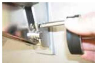
**Figure 2-28. Swim Step Pin Removal**
