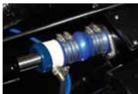
**Figure 4-7. Drip Less Shaft Packing**
