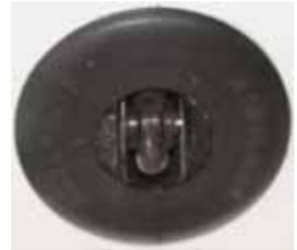
Figure 2-35. Thru-Hull Paddle Wheel Pickup
