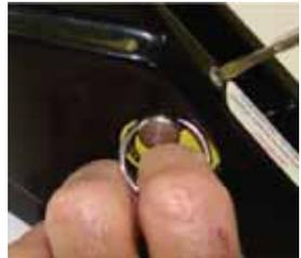
7. If you suspect ball plunger is not holding locking pin correctly, it will be necessary to remove ball plunger and inspect working end of plunger.
