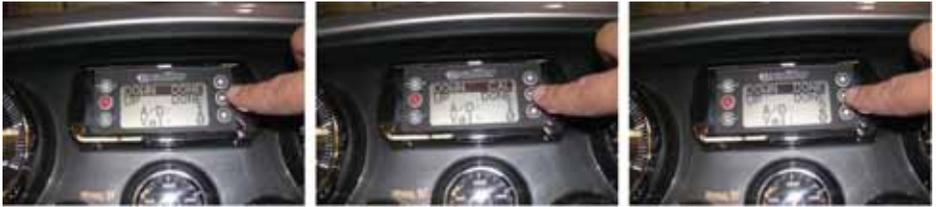
4. Now you will need to raise the Wedge “all the way up.” (MMDC must see 1 MPH before it will let the Wedge come up.) Once you are sure the Wedge is all the way up, scroll the cursor over “UP.” With “UP” highlighted, press “E.” Wait 2 seconds and press “E” again. The Power Wedge is now calibrated. Press the RED button several times to get back to the main screen.
