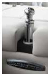
**Figure 2-26. Pivoting-Head Ski Pylon**
