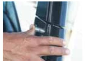
5. Be sure the rings on both quick-release pins are in the locked position before operating the boat.
