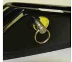
2. Insert locking pin all the way into lower base.
