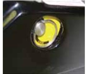
3. Screw ball plunger all the way down by turning clockwise until it stops.
