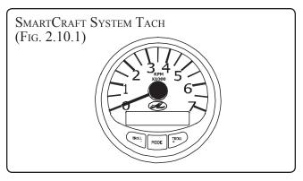
Your boat is equipped with the SmartCraft<sup>TM</sup> instrumentation system. The SmartCraft<sup>TM</sup> system consists of a smart tachometer with a display screen.
