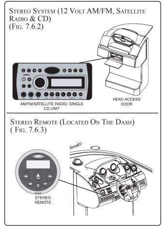
The stereo is protected by the stereo fuse on the bilge component board. The power source and fuse protection for the stereo memory is on the bilge component board. Power to stereo memory is maintained even if the battery switch is off.
