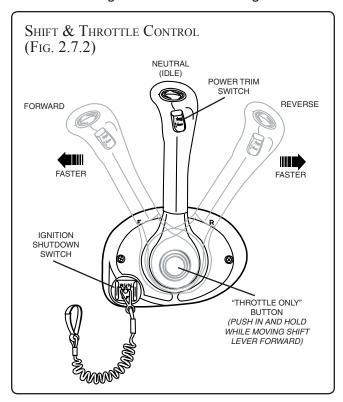
The "throttle only" mechanism may differ from one style shift/throttle unit to another. Refer to your Gear Shift & Throttle Manual for proper operation of this feature.
