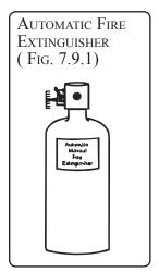
Your boat may be equipped with an automatic fire extinguisher system located forward of the engine. In the event of a fire, the heat sensitive automatic head will release the extinguishant as a vapor, totally flooding the area in fire-killing concentrations.
