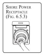
the locking ring onto the boat receptacle to prevent accidental unplugging.
