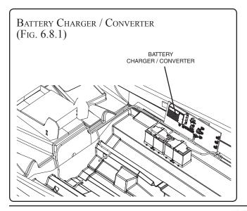
**Note**: Leave the charger/converter turned ON at all times to maintain battery voltage level.
