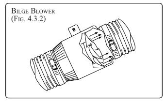
The bilge blower is protected by a fuse on the accessory fuse block located at the helm (See Fig. 6.3.1).
