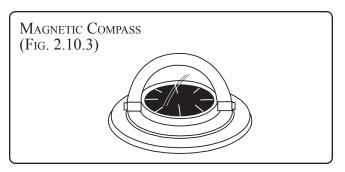
Your compass, properly corrected, will indicate magnetic north (not true north). A compass must be adjusted by a qualified person. The reason for this is that nearby instruments or objects containing magnets or current-carrying electrical wires will influence the compass reading. This is especially true if you add electronic devices to the helm station.
