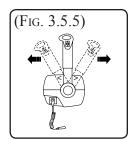
do not shift quickly from neutral into gear. Once clear of the dock, mooring, people and/or the no-wake zone and the boat has been shifted into forward gear, move shift/throttle lever forward to desired engine speed.
