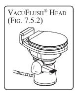
The VacuFlush® head utilizes a HEAD SYSTEM breaker on the main distribution panel. The foot pedal at the base of the toilet opens a mechanical seal and vacuum forces waste through the opening in the bowl to an accumulator tank, through the vacuum pump and then
