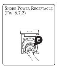
F. Clean the power cord, spray the cord ends with moisture repellent, and store the cord in a dry location on board.
