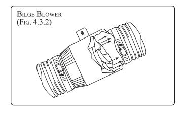
The bilge blower is protected by a fuse on the accessory fuse block located behind the access panel above the MDP in the STBD storage area (See Fig. 6.3.1).
