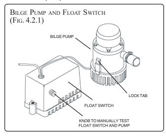
If the liquid level in the bilge is higher than normal and the bilge pump empties the bilge when you use the ON switch, either the breaker for the automatic bilge pump circuit has blown or the float switch is not operating properly. Have it checked immediately. If the ON switch does not operate the pump, DO NOT use the boat until the problem is corrected.
