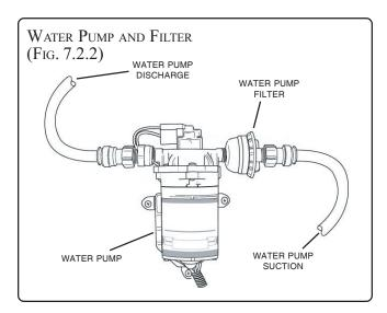
The water pump and filter are located on the port side of the engine room above the water heater. The filter prevents particles from entering the pump head. The filter should be checked and cleaned once a season or when flow is restricted.
