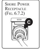
receptacle. Turn clockwise to lock. Thread the locking ring onto the boat receptacle to prevent accidental unplugging.
