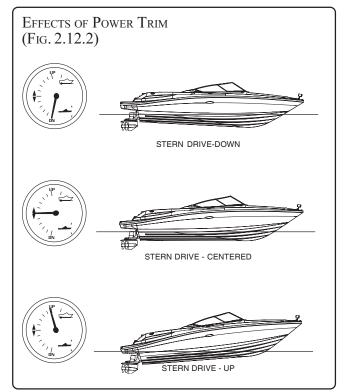
If you raise the stern drive up too far while you are on plane, you could cause a loss of speed and power due to condition called propeller "ventilation." If this happens, there will be a sudden increase in engine RPM and loss of speed. Do not let this condition exist. Immediately reduce your engine RPM and trim the outdrives DOWN slightly until engine slows down and you regain forward speed.
