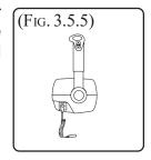
Then move shift/throttle lever rapidly, either forward or reverse, but not very far from the neutral position. The drive unit will engage and boat will start to move slowly in either forward or reverse. You can damage the transmission if you
