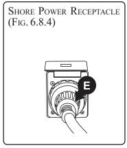
F. Clean the power cord, spray the cord ends with moisture repellant, and store the cord in a dry location on board.
