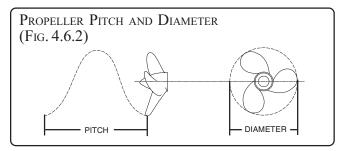
Propellers have two basic characteristics:
