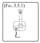
throttle. In cold weather, it may be necessary to pump lever several times before engine will start.
