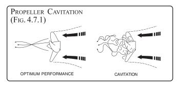
Cavitation is a phenomenon that occurs in all propeller-driven craft under certain conditions. The surface of propeller blades are not perfectly flat, and as water is drawn through the blades to be discharged aft into the propeller's slip stream, the water flowing over the curved surface of the blade encounters areas of greater and less pressure.
