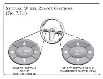
**The SOURCE buttons group** controls the stereo system.
