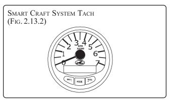
Your boat is equipped with the SmartCraft<sup>™</sup> instrumentation system. The SmartCraft<sup>™</sup> system consists of a smart tachometer with a display screen.
