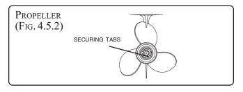
2. Straighten the bent tabs on the propeller nut retainer (Figure 4.5.2).
