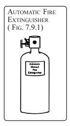
Your boat may be equipped with an automatic fire extinguisher system located forward of the engine. In the event of a fire, the heat sensitive automatic head will release the extinguishant as a vapor, totally flooding the area in fire-killing concentrations.
