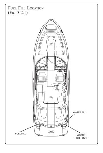
Open fuel fill cap and insert hose nozzle into the fuel fill opening. Fuel fill hose nozzle must contact the fuel fill opening BEFORE adding fuel, and throughout the fueling process, to prevent discharge of static electricity.
