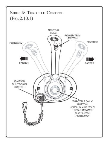
Shift/throttle controls are equipped with a "throttle only" mechanism which allows the shift mechanism to be disengaged from the throttle. This allows the throttle to be advanced without shifting the transmission when starting. It may be necessary to use the "throttle only" button in order to pump fuel into the engine for ease in starting.
