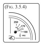
IF ENGINE TEMPERATURE GOES ABOVE NORMAL RANGE SHUT DOWN THE ENGINE IMMEDIATELY. GET TRAINED HELP TO FIND AND FIX THE PROBLEM.
