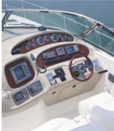
*At the helm, the captain enjoys a wood-accent tilt wheel with hydraulic steering and dual gear shift and throttle controls.*
