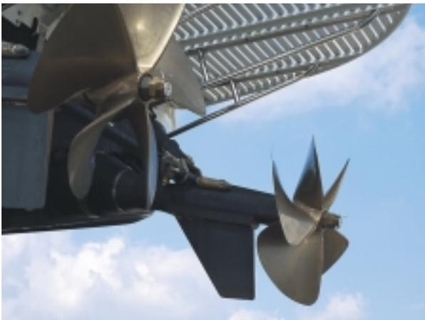
*Twin Arneson ASD12 surface drives, in concert with powerful twin diesel engines and the stable, wide beam, help captains conquer any waters easily.*
