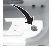
there is a cap that is tethered to the fitting which should be ON THE CONNECTION when it is not in use.
