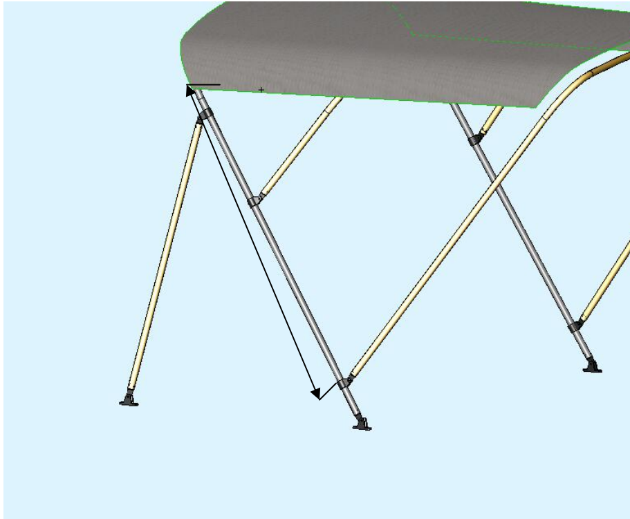
Figure 2- Measure from jaw slide to side line on both sides.
