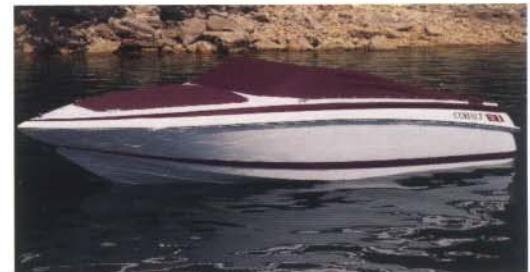
Tonneau Covers - bow and cockpit covers shown. Not recommended for long term storage
