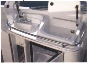
Cockpit Galley Unit
