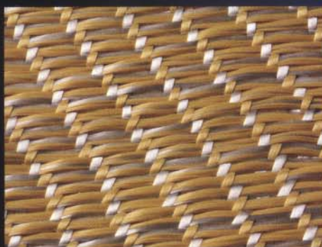
Kevlar®/E-glass knit material
