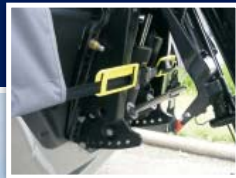
Stern Protector Pads guard against possible chaffing from connector straps
