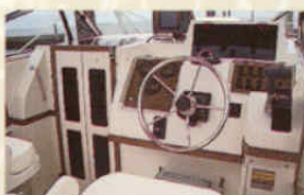
Helm station with lockable electronics box
