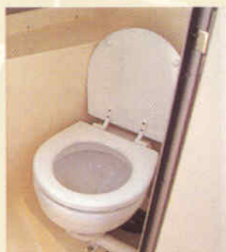
▲ Marine head with holding tank
