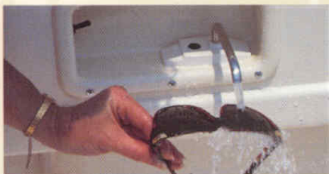
▲ Gunwale mounted freshwater system
