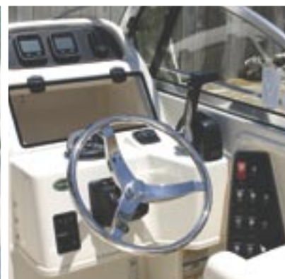
Helm station with lockable electronics box
