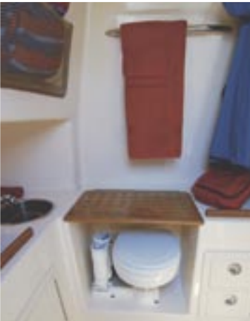
Lockable head enclosure with fold down cover, sink and storage
