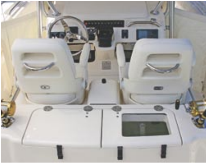
Command seating helm area with two deluxe adjustable sliding chairs and rigging station with freshwater sink, pullout faucet and insulated livewell
