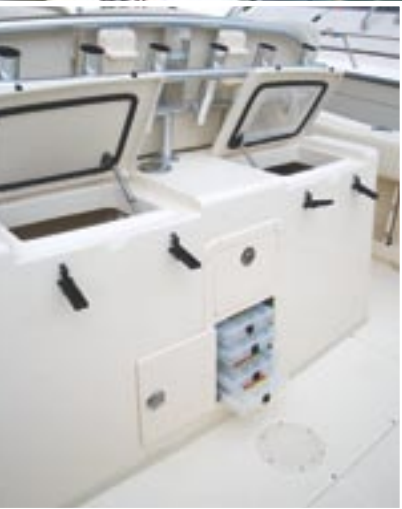
Rigging station with freshwater washdown, 104-qt. cooler, tackle drawers, storage, rod holders and knife & pliers holders
