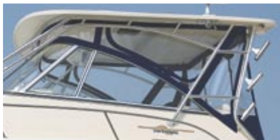
▲ Hardtop front and side curtains for models 20' and up (330 shown). Drop curtain is available. Frames style and canvas vary per model.
