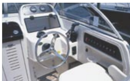
Helm station with lockable electronics box
