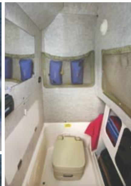
Lockable stand up console head enclosure w/storage shelves and hanging locker; shown with optional portable head
