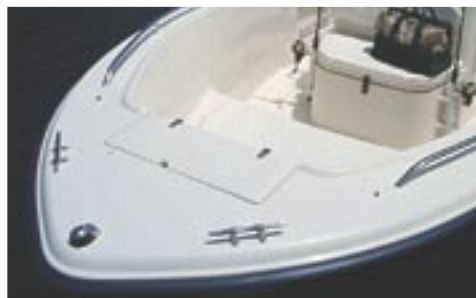
Forward console with seating and bow anchor locker
