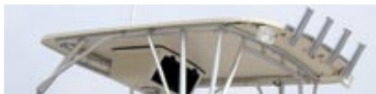
▲ Hardtop with lockable radio box, spreader lights and rod holders (208)
