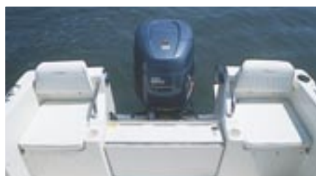
Aft cockpit with fold down motorwell bulkhead
