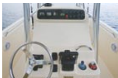
Helm with flush mount electronics area
