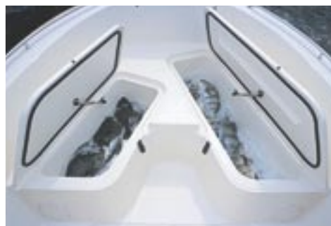
Insulated bow fish boxes with overboard drains
