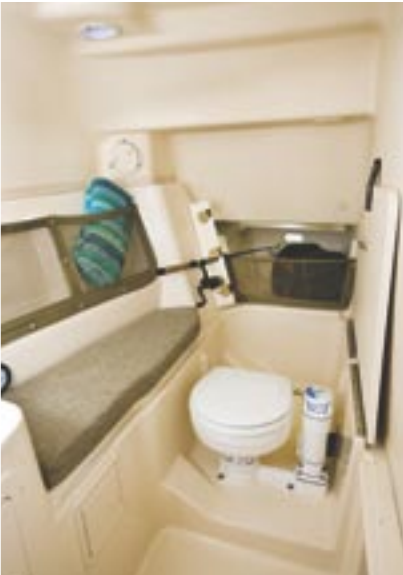
Stand up head area with bulk storage; fold down head cover creates 5' berth.
