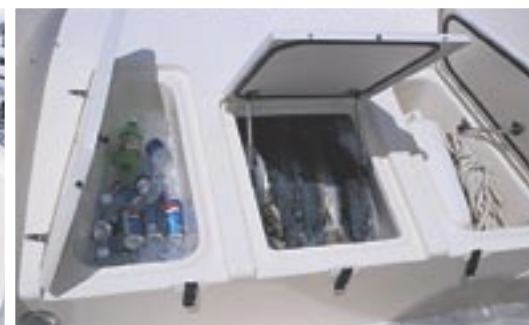
Insulated bow fish boxes with overboard drains
