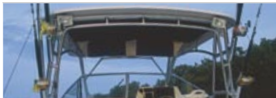
▲ Hardtop with lockable radio boxes, spreader lights, side rod holders and overhead storage net (optional for cabin models 22'-25', standard for 29'-36')
