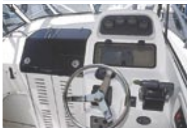
Helm station with lockable electronics box
