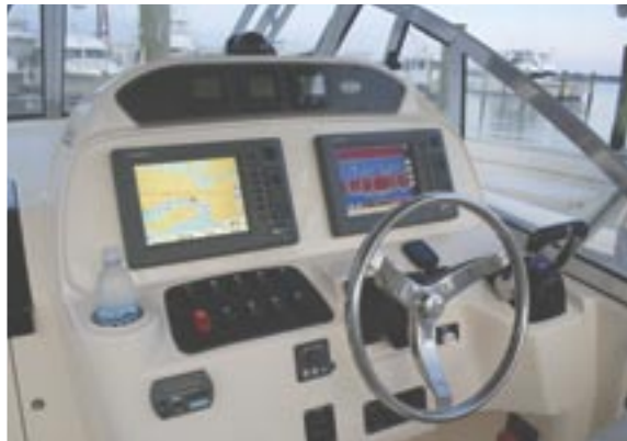
Helm with flush mount electronics
