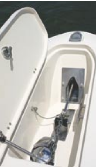
Anchor locker with windlass
