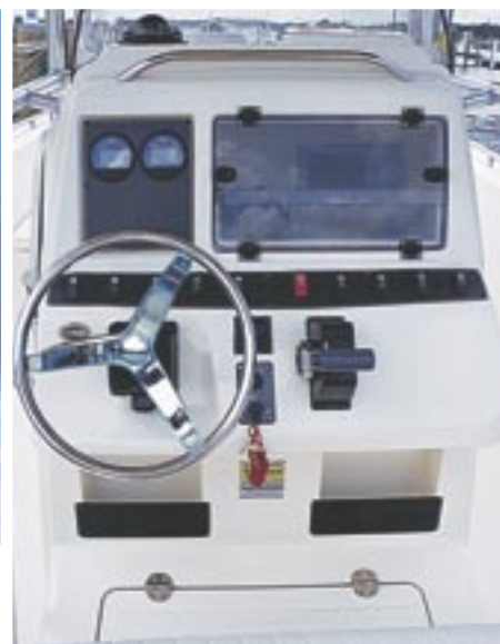
Helm station with lockable electronics box
