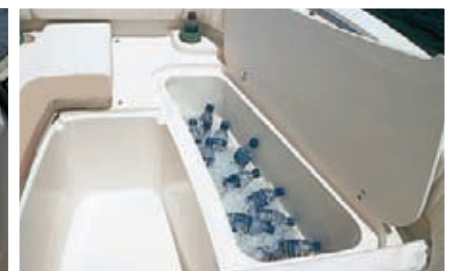
Forward seating with insulated fish box
