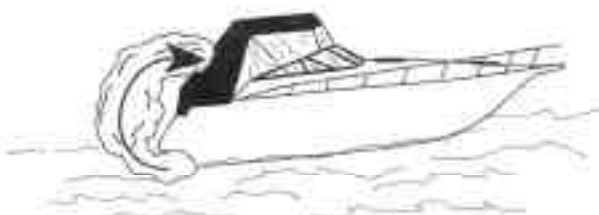
FIGURE 2.3 CO ACCUMULATION WITH PROTECTIVE COVERINGS
