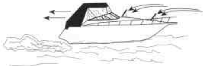
FIGURE 2.5 OPERATION AT SLOW SPEED AND PROPER VENTILATION
