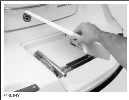
F14L1HY LIFT LADDER COVER UNTIL STOPPED BY RETAINING SPRING (SPRING NOT SHOWN)
