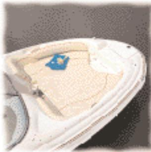
In the bow, a concealed swim ladder gives easy access to the water or shore, while the roomy seating area provides storage beneath the cushions. A hi-lo table can adjust to support a sun pad filler cushion.
