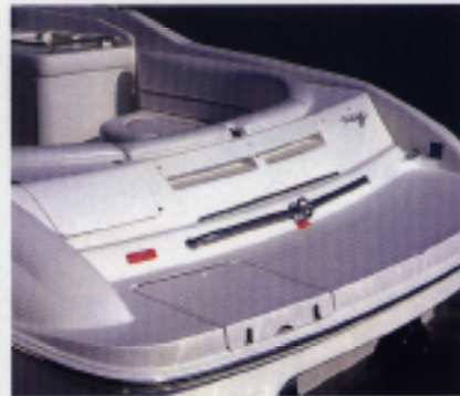
The large swim platform provides a hatch for concealing the swim ladder, easing entrances and exits.
