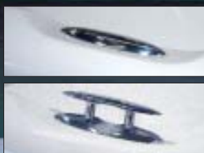
Stainless steel pull up cleats retract to clear the deck.
