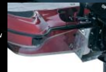
Ladder remains hidden when not in use: When closed, the ladder appears as nothing more than a recessed handle below the rub rail
