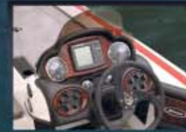
New Console: Ergonomic floating console with oversized racing gauges for improved readout.
