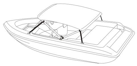
10 It is much easier to install the assembled bimini with two people, one to hold each side while positioning it onto mounts. Secure bimini to mounts with screws provided. Adjust hold down straps and bow straps to achieve desired tightness. If you have any questions or additional parts are needed for your specific boat application, please call (800) 874-6824.
