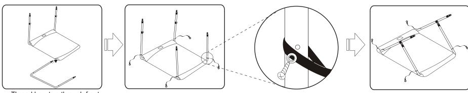
Thread bow two through front sleeve of fabric. Holes in bow should face toward the center of fabric.
