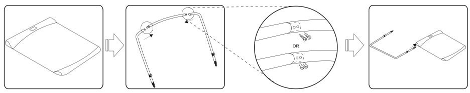
Lay bimini fabric face down on a flat surface (label on rear sleeve will be facing up).
