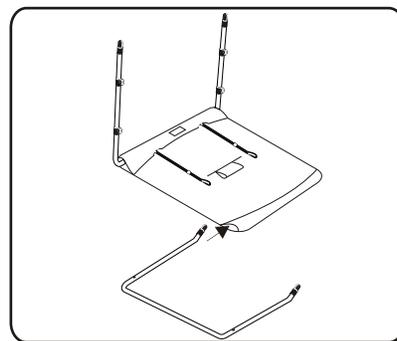
**6** Thread bow two through front sleeve of fabric. Holes in bow should face toward the center of fabric.
