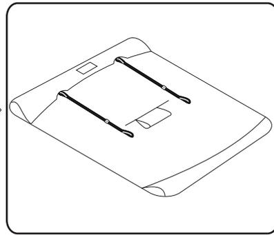
**2** Insert bow straps into cutouts of rear sleeve as shown.
