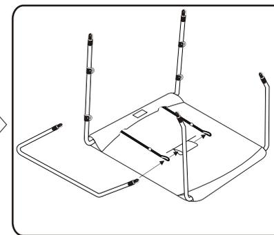
**7** Thread bow three through middle sleeve and bow strap loops.
