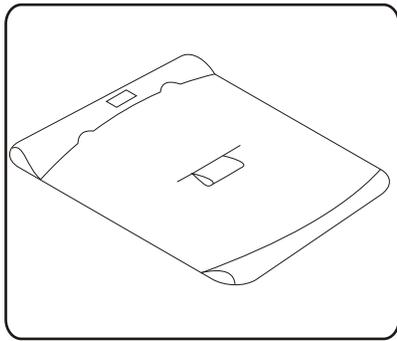
**1** Lay bimini fabric face down on a flat surface (*label on rear sleeve will be facing up*).
