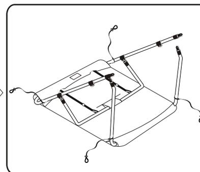
**10** Connect third bow end to lower jaw slide of bow one and secure with screws.
