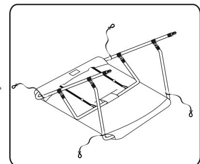
**11** Connect ends of second bow to upper jaw slides of bow one and secure with screws.
