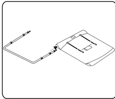
**5** Thread bow one through rear sleeve and bow strap loops. Jaw slides will face toward center of fabric.
