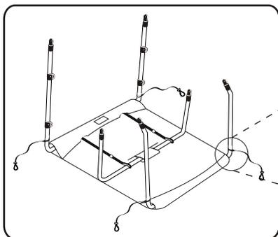
**8** Pass looped end of hold down strap over end of bow. Repeat for bow ends shown. . .
