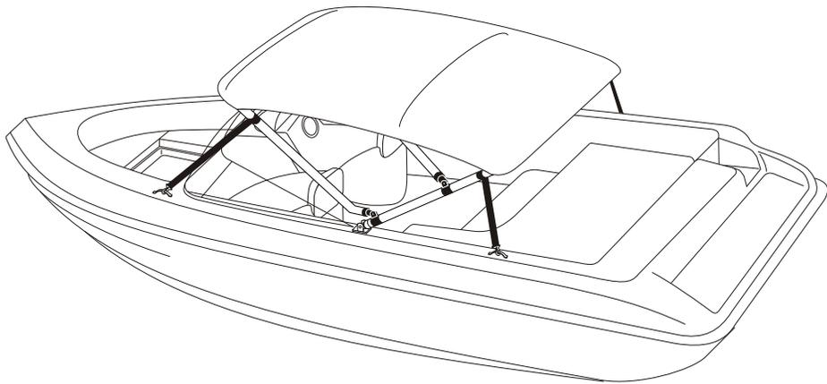
**13** It is much easier to install the assembled bimini with two people, one to hold each side while positioning it onto mounts. Secure bimini to mounts with screws provided. Adjust hold down straps and bow straps to achieve desired tightness. If you have any questions or additional parts are needed for your specific boat application, please call (800) 874-6824.
