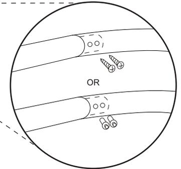
**4** . . . and inserting screws as shown (if hammer rivets, tap firmly with hammer to set). Repeat steps 3 and 4 for other bows.
