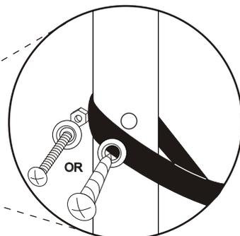
**9** . . . and secure front straps with screws. Rear straps use nuts and bolts.
