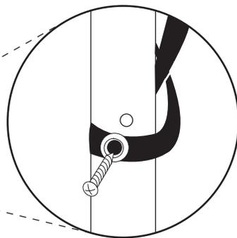
**9** Line up hole in each strap with the hole in the bow. Insert #8x5/8" screw through washer and strap, and secure into bow. Strap should extend away from the top. Repeat for remaining bow straps.
