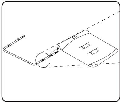
**4** Position Bow 1 as shown with jaw slides facing up. Thread Bow 1 thru rear sleeve.
