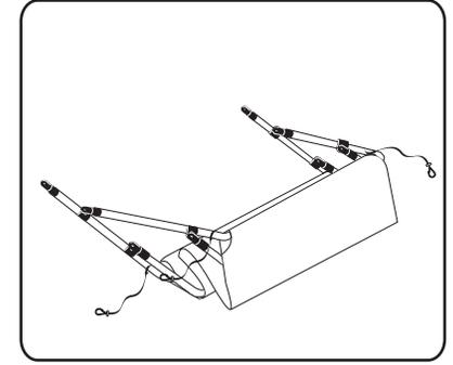
**11** Remove screws from remaining jaw slide of Bow 1. Thread screw through jaw slide and Bow 2 eye end and secure to connect. Eye ends will rotate to line up.
