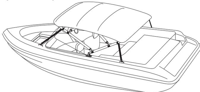
**13** With bimini secure in the mounts, open the bimini and determine the best position for the hold down strap eyes. Strap eyes should be mounted to a flat surface whenever possible and straps should maintain an angle between 30 and 60 degrees from front to rear. To minimize side to side movement, it is suggested to mount front strap eyes as far inboard as allowable. Line up strap eyes across the boat.
