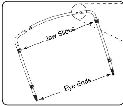
**1** Assemble pieces of Bow 1 by attaching both Bow 1 sides to the Bow 1 center.
