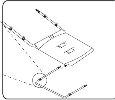
**5** Position Bow 2 as shown with holes facing up. Thread Bow 2 through front sleeve of fabric.
