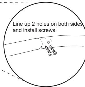
**2** ... and inserting 5/8" screws as shown. Repeat steps 1 and 2 for other bows.
