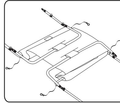
**10** Remove screws from Bow 1 jaw slide nearest to Bow 3. Thread screw through jaw slide and Bow 3 eye end and secure to connect pieces. Eye ends will rotate to line up. Repeat steps above with Bow 2 and Bow 4.
