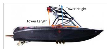
Fits boats with the tower mounted over the windshield with the top of the tower not to exceed 24" behind the wing of the windshield. Max tower height from top of gunnel: 68". See diagram.
